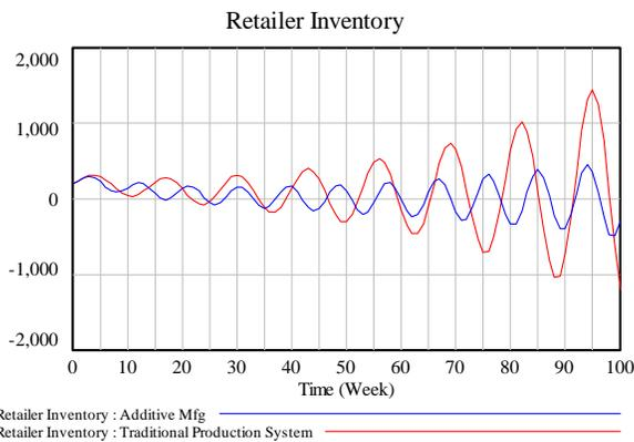
**Figure 7.** The trend of retailer's inventory over time in both AM and traditional systems (stronger pipeline effect in traditional manufacturing)
