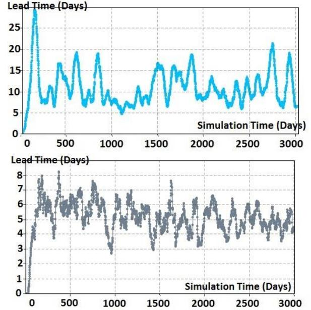
Figure 5. Lead time in the classic supply chain (Scenario 1, top graph) and AM supply chain (Scenario 2, bottom graph)
