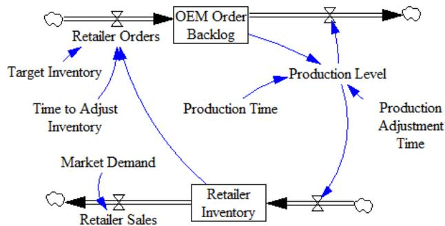
**Figure 6.** Stock and Flow diagram for retailer's ordering procedure (Modified from [34]).
